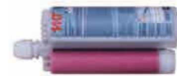
Cartridge VME 385 Side-by-side cartridge Content: 385ml With big mixer VM-XL and reducers / extension tube for drill holes from 12mm diameter
