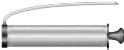
Blow-out pump (volume 750ml) Drill bit diameter (d 0 ): 10 mm to 20 mm Drill hole depth (h 0 ): ≤ 10 d nom for uncracked concrete
