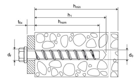
$\begin{array}{llll} d_0 & = & \text{nominal drill hole diameter} \\ h_{\text{nom}} & = & \text{nominal embedment depth} \\ h_1 & = & \text{depth of the drill hole} \\ h_{\text{min}} & = & \text{minimum thickness of member} \\ t_{\text{fix}} & = & \text{thickness of fixture} \end{array}$
